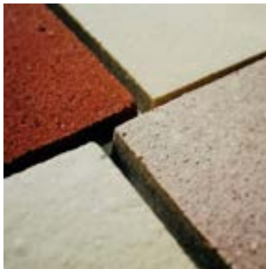
StoneCycling Waterproofing Tiles. Demolition waste. Tom van Scest, The Netherlands.
