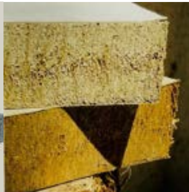
Enviro Board Insulating Panels. Straw waste. Enviro Board Corp, NJ, USA.
