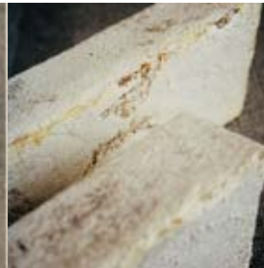
Mushroom Bricks Construction Bricks. Mycelium, straw waste. The Living, NY, USA.
