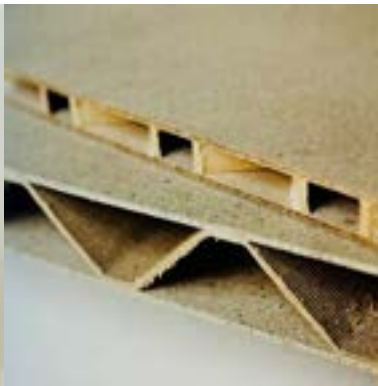
ECOR Construction Panels. Waste materials with high fibres. Noble Environ. Tech, CA, USA.
