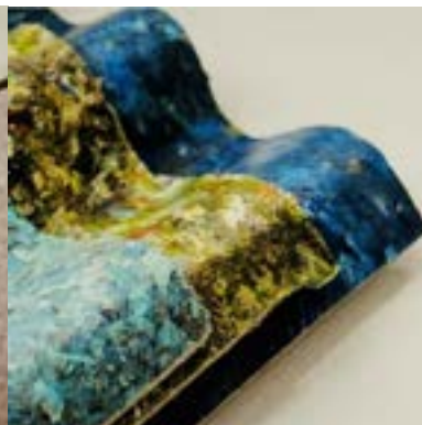
Tuff Roof Waterproofing Panels. Discarded Tetra Pak cartons. Deman Ganga Paper Mill, India.
