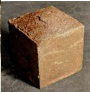
Blood Bricks Construction Bricks. Discarded animal blood and sand. Munro, UK.
