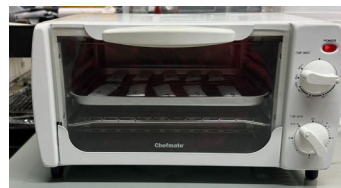
Figure 4- Chefmate T0-09 1000 watt Toaster Oven with stationary pan Conditions: 150 F, 3 hours
