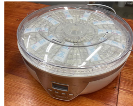
Figure 2- Ambiano 95459 Food Dehydrator with circular grated platforms and low humidity heated air from base. Conditions: 150 F, 10% RH, 3 hours
