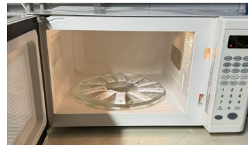
Figure 3- Chefmate P70D20AL-D4 1050 watt Microwave with rotating glass plate Conditions: 10-70% power, 15 min
