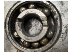
Removal with Dremel of inner race & rollers
