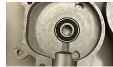
Bearing before removal
