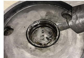
Bearing removed of the inner race & rollers
