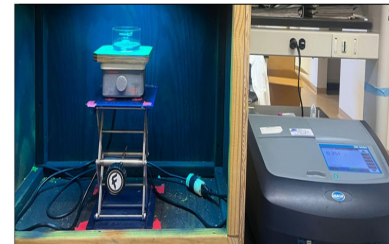
Figure 1: AOP Set Up (Spectrophotometer on the right and UV lamp with water sample on the left)
