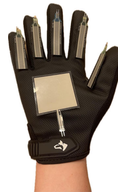
Figure 4. Prototype Assembly of Flexible Pressure Sensing Glove
